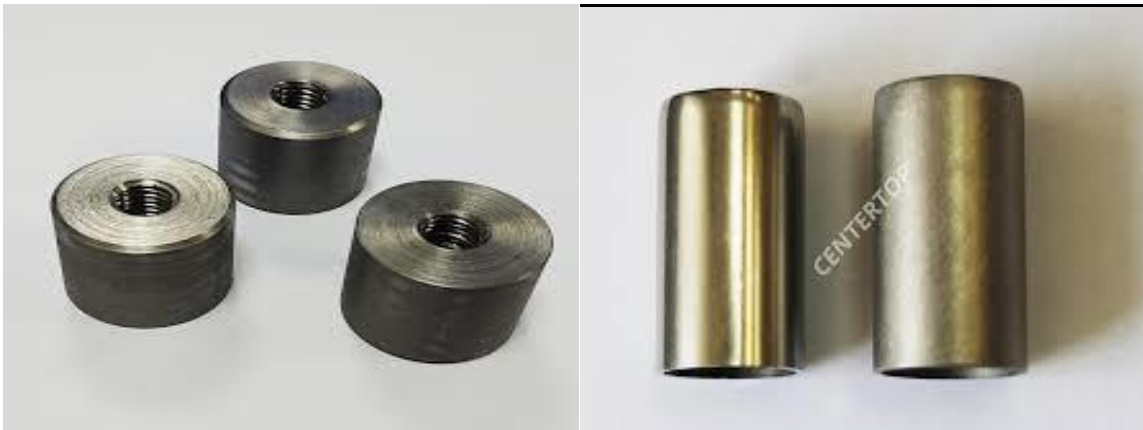
Before and after turning
