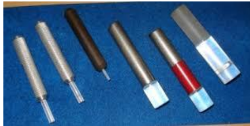
Gauge - smooth plug with handle for small diameters - 426DS
