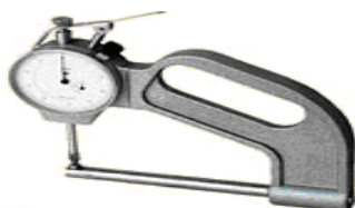
Indicator thickness gauges for measuring walls of parts.
