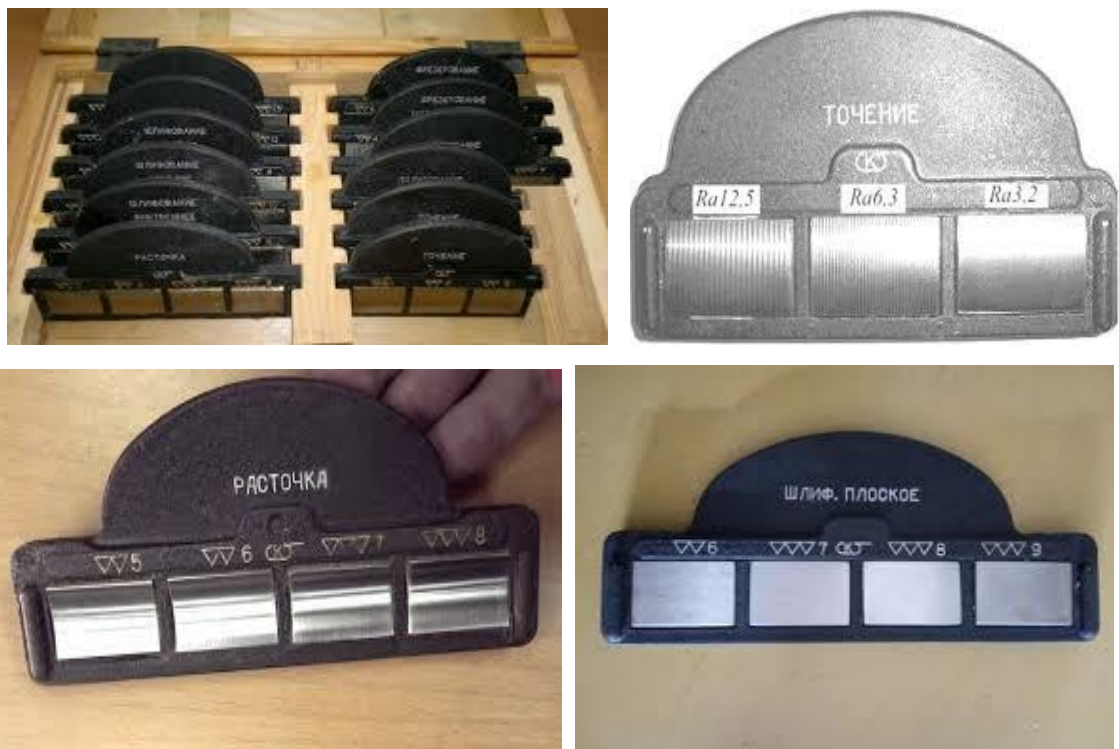
Samples of surface roughness after different technological operations
