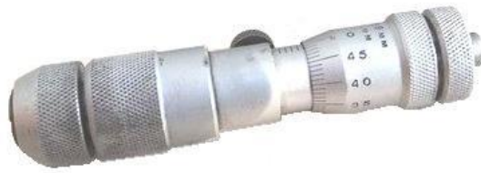
Internal micrometer NM 75-0.01 GOST 10-2000
