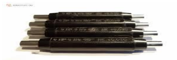
Caliber plug smooth D5H9 PR = 0 NE = +0
