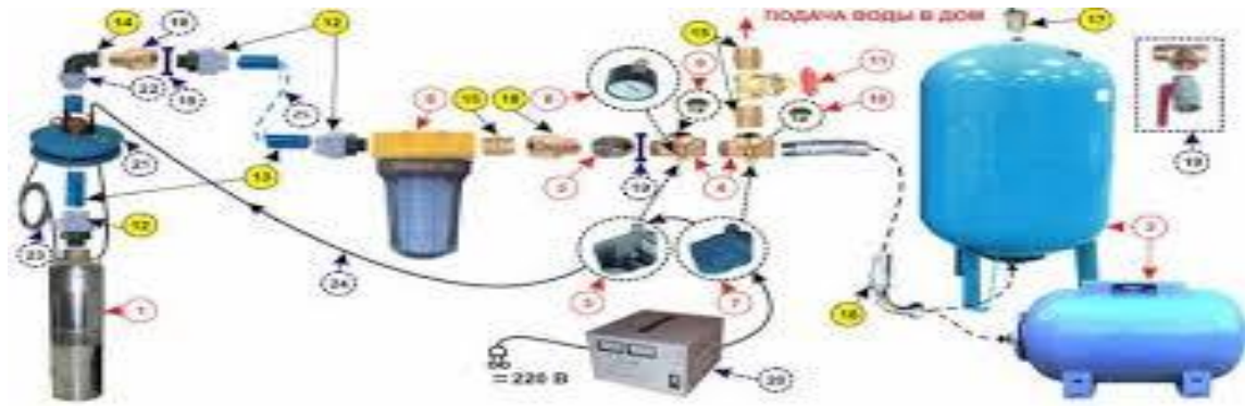
Connection diagram of a well pump with a relay
